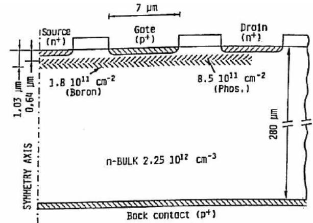
Fig. 1. Cross-section of the SSJFET. The conductive channel is obtained by a deep phosphorus implant. The substrate is high resistivity n-type silicon.
