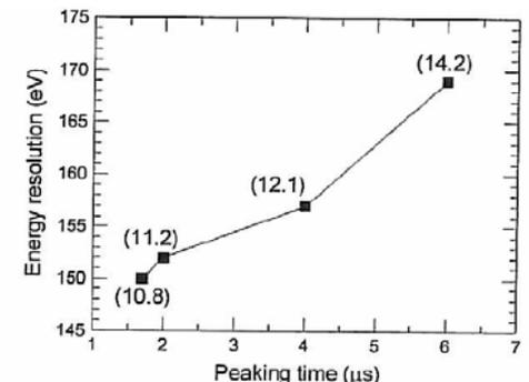
Fig. 14. Energy resolution measured at the Mn-K $\alpha$  line at the four different peaking times. The corresponding value of electronics noise (in electrons rms) is reported for each measurement.
