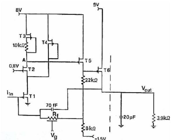
Fig. 10. Circuit diagram of the charge sensitive preamplifier.
