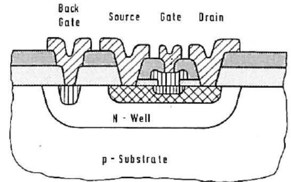
Fig. 11. Cross section of the JFET compatible with CMOS-bipolar technology.
