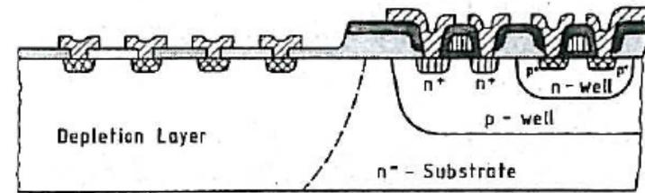
Fig. 15. Junction isolation of monolithic silicon detectors and readout electronics
