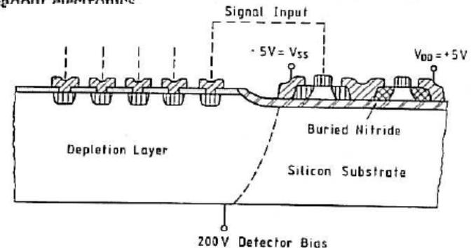
Fig. 19. Isolation scheme of silicon detector and buried nitride technology for readout electronics.
