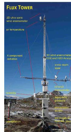
Figure 5. Micrometeorological tower with eddy covariance instrumentation installed at Finse in 2016.
