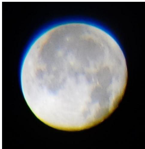
Figure 10: Chromatic aberration as seen when observing the Moon through a refracting telescope.
