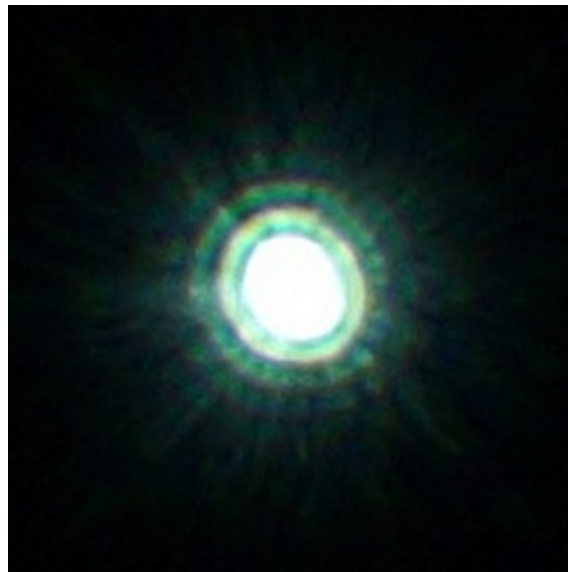
Figure 14: Airy disks around a star, representing the limitations because of the diffraction pattern of light passing through a circular aperture.
