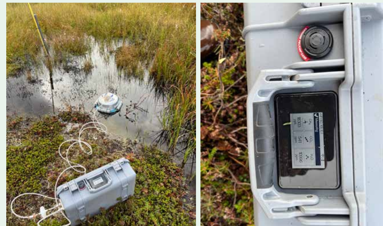
Figure 4: Floating chamber connected to Licor (Li-7810) (left) and values measured (right).
