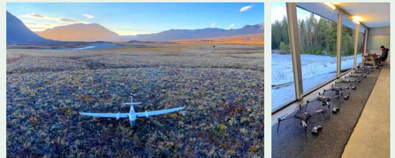
Figure 2: Current detector hardware, operated by the DroneLab core facility at the Department of Geosciences. Left: Commercial vertical-takeoff-and-landing drone "Trinity F90" with meteorological sensors tested near the Zackenberg Ecological Research Station, North-East Greenland, in August 2022. Right: "UiO-Flamingo" multi-copter drones for swarm applications at a test site near Oslo.
