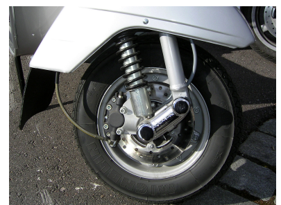
Figure 3.4 Front suspension of a classic Vespa scooter showing a shock absorber and a spring in a coilover configuration (“coil spring over shock”) to the left. The structure to the right is a swing-arm. Image: Public domain, from Wikipedia Commons. ( Wikipedia )
