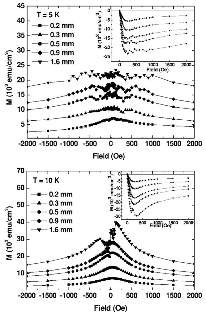
FIG. 2. Magnetization hysteresis loops  $M(H)$  for  $\text{MgB}_2$  films with different widths at 5 (a) and 10 K (b). The noisy region around  $H=0$  is a result of dendritic flux avalanches. Inset: the virgin branches of the loops.
