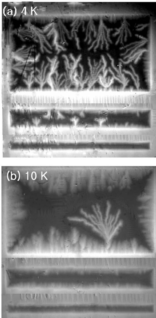
FIG. 1. Magneto-optical images of flux penetration into the virgin state of  $\text{MgB}_2$  thin films with widths of 1.6, 0.4, and 0.2 mm at  $T=4$  (a) and 10 K (b). Numerous dendritic structures were formed by abrupt flux avalanches. The applied field is 18 mT.
