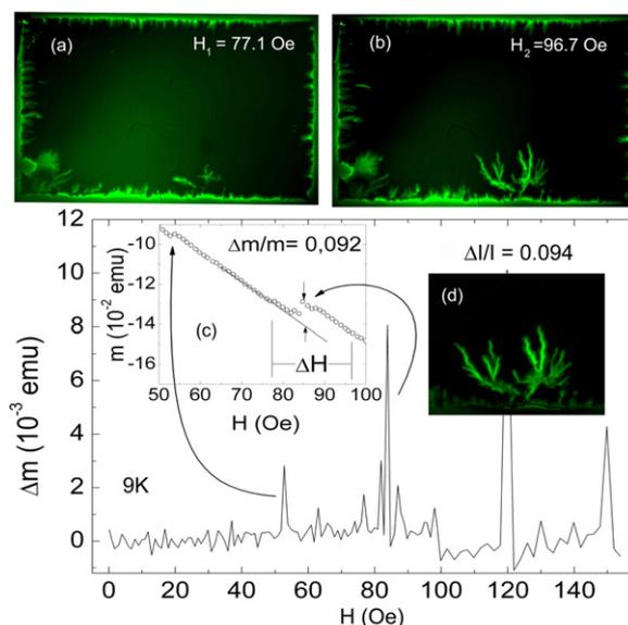
**Figure 2.** Main graph shows difference between successive values of the magnetic moment measured at 9 K. Images (a) and (b) were taken at the fields indicated, corresponding to the same  $\Delta H$  shown at the original  $m(H)$  curve, inset (c). Inset (d) is the difference in intensities, (b) minus (a).
