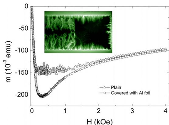
**Figure 1.**  $m(H)$  taken at  $T = 4$  K for a plain  $\text{MgB}_2$  film (fluctuating) and for the same sample covered with a piece of aluminum foil (smooth). Inset: MOI taken at 4 K and 120 Oe of a similar  $\text{MgB}_2$  film half-covered with Al foil.
