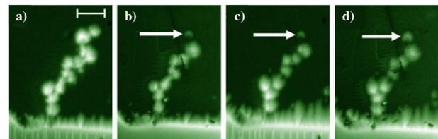
**Figure 8.** MO images of the same *ex situ* film during four different sets of measurements; the applied field is about 10.2 mT and the temperature is 4 K for images (a) and (b), 8 K for image (c) and 15 K for image (d); the scale bar corresponds to 0.2 mm. The arrow marks a ‘run-away’ flux spot.
