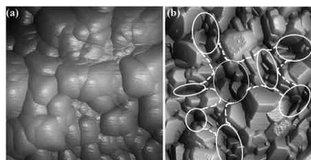
**Figure 5.** AFM pictures of (a) the *in situ* and (b) the *ex situ* films; the areas covered are  $0.5 \times 0.5 \mu\text{m}^2$  and  $2 \times 2 \mu\text{m}^2$  respectively; the white circles in (b) correspond to incomplete holes on the surface of the film and the dashed lines to shallow valleys.
