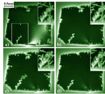
**Figure 7.** MO images of the same *ex situ* film during four different sets of measurements. The applied fields are (a) 10.2 mT, (b) 8.5 mT, (c) 10.2 mT, and (d) 11.9 mT. All the pictures were taken at  $T = 4$  K. The insets show the area corresponding to the area marked by the white rectangle in figure (a) for the same set of measurements respectively but at higher fields ( $H_a = 34$  mT).
