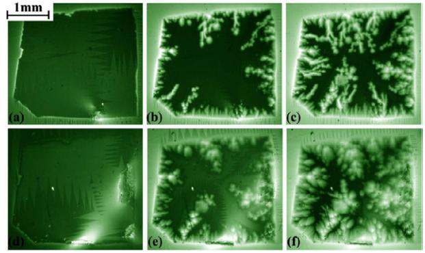
**Figure 2.** Magnetic flux penetration in the *ex situ* film: (a)  $T = 4$  K,  $H_a = 3.4$  mT, (b)  $T = 4$  K,  $H_a = 17$  mT, (c)  $T = 4$  K,  $H_a = 25.5$  mT, (d)  $T = 15$  K,  $H_a = 3.4$  mT, (e)  $T = 15$  K,  $H_a = 17$  mT, (f)  $T = 15$  K,  $H_a = 27.2$  mT. The bright region in the lower right corner is due to stress in the indicator film and do not correspond to a high magnetic flux density area.
