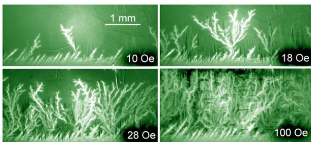
FIG. 2. (Color online) Magneto-optical images of flux distribution in a 0.29  $\mu\text{m}$  thick NbN film at 3.5 K for increasing magnetic field. The image brightness represents the magnitude of the local flux density.
