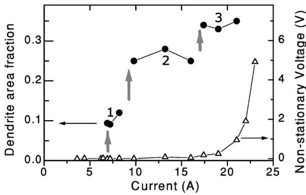
FIG. 3. The area covered by the current-induced dendrites (solid circles) at  $T=12.5$  K. The vertical arrows indicate at which currents the number of dendrites increases by one. Open triangles show an increase in the voltage from 1.0 to 2.7  $\mu$ s after the pulse start.
