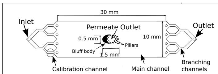
(a) The hydrodynamic particle separation microchip. The trilobite shaped separation unit is located in the center of the channel. Channel height is  $90 \mu\text{m}$ . Inlet and permeate outlet are pressure regulated. The outlet downstream is an atmospheric pressure outlet. Permeate outlet, pillars and bluff body not to scale.
