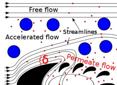
(b) Working principle of the trilobite shaped separation unit: Large blue particles can be separated from the small particles even when inside  $\delta$  because they have different inertia.
