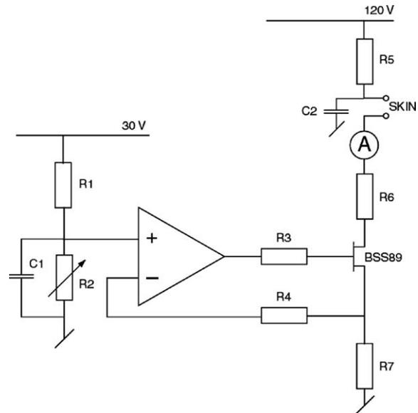
Fig. 1. Electronic constant current source.
