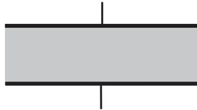
**Figure 4.** The basic capacitor model.
