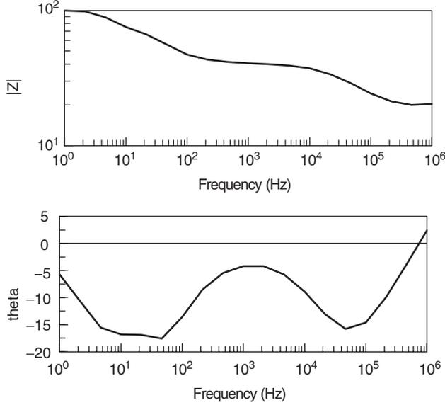
**Figure 2.** Typical impedance spectrum obtained with four equal electrodes attached to the skin of the underarm as shown on Fig. 1 (right). All electrodes are pregelled ECG-electrodes with skin gel-wetted area  $3\text{ cm}^2$ . Distance between electrode centers: 4 cm.
