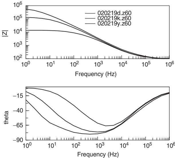
**Figure 3.** Typical impedance spectrum obtained with the 3-electrode system on the underarm as shown on Fig. 1 (middle). The parameters are: at the time of electrode onset on dry skin, after 1 h, and after 4 h of contact.
