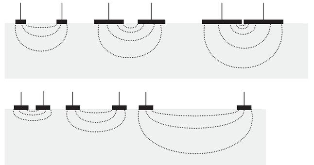
**Figure 7.** The measuring depth as a function of electrode dimensions (top) and electrode spacing (bottom). From (2), by permission.
