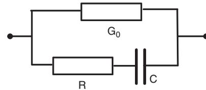
Figure 10. Tissue or suspension equivalent circuit.
