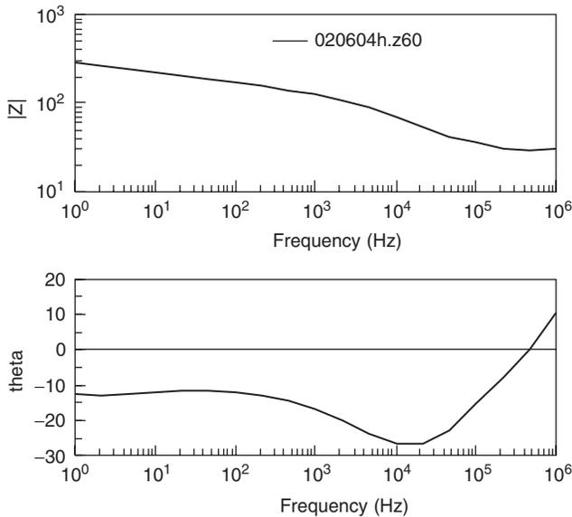
**Figure 11.** Electrode polarization impedance, one pregelled ECG commercial electrode of the type used in Figs. 2 and 3. The positive phase at HF is caused by the self-inductance of the electrode wire.
