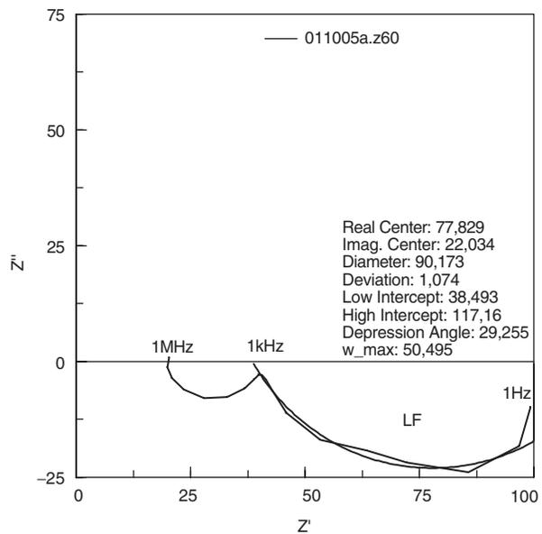
Figure 9. The data in Fig. 2 shown in the complex Wessel diagram as  $Y$  and  $Z$  plots. Circular arc fits for the same LF dispersion are shown in both plots.
