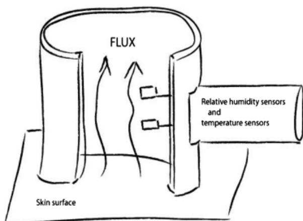
Fig. 1. Illustration of the measurement principle, Tewameter TM 300.
