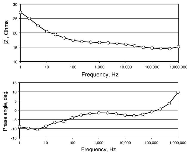
**Figure 10.** Four underarm skin surface electrodes with 4 cm centre separation. Each electrode 3 cm<sup>3</sup> gel wetted area.
