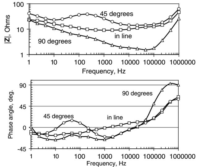
**Figure 5.** Transfer impedance found with skin surface PU electrodes oriented parallel, oblique  $45^\circ$  and perpendicular to the presumed current density direction.
