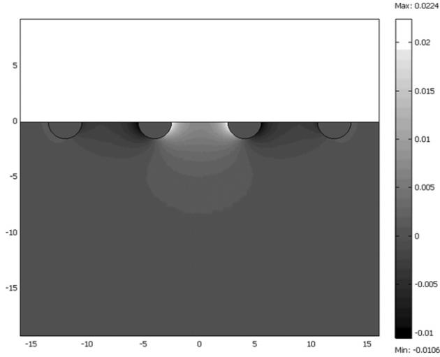
**Figure 1.** Sensitivity distribution of a tetrapolar electrode system.
