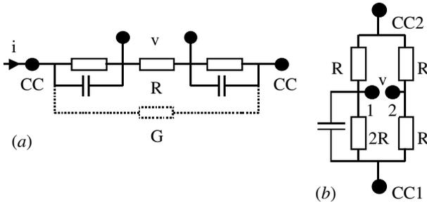
**Figure 3.** Simple four-terminal, two-port networks. (a) Single series current path, with second path stippled. (b) Bridge.
