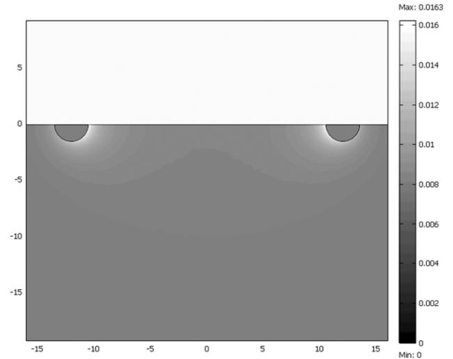
**Figure 2.** Sensitivity distribution of a dipolar electrode system.
