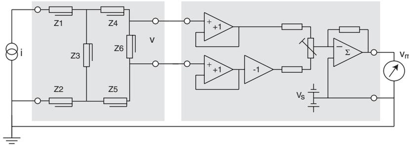
**Figure 8.** Equivalent circuits for tissue and a potential amplifier. The impedance symbol is for frequency dependent components.
