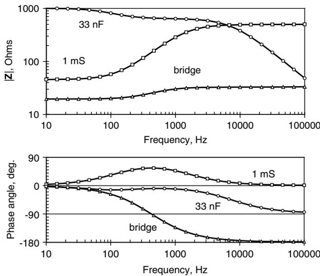
**Figure 4.** Bode plot for the networks of figure 3. Component values:  $R = 1 \text{ k}\Omega$ , parallel combination  $10 \text{ k}\Omega$  and  $0.1 \mu\text{F}$ ,  $G = 1 \text{ mS}$  or  $C = 33 \text{ nF}$ . Bridge:  $R = 100 \Omega$ ,  $C = 2.3 \mu\text{F}$ .
