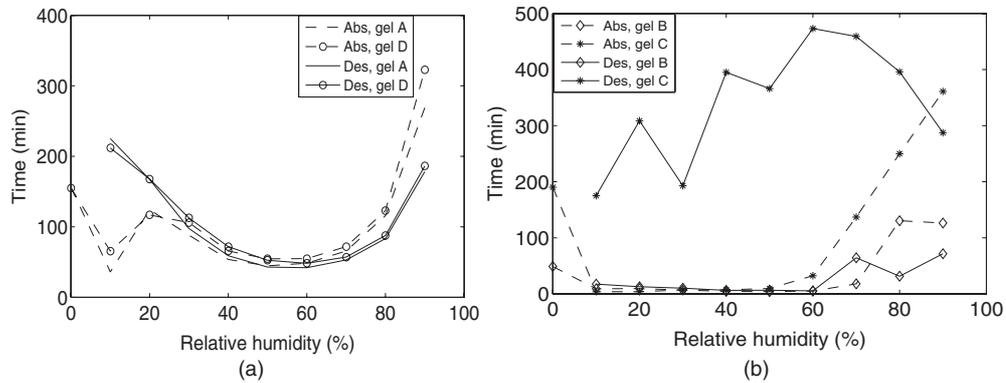
**Figure 4.** Time constants for gels A and D in (a) and B and C in (b). The points to the far left in the graphs illustrate the characteristic time for the gels to reach equilibrium with the dry chamber, starting from their initial hydration state.
