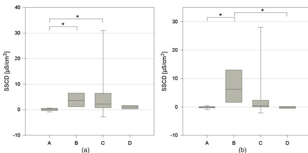
**Figure 6.** Quantization of the pressure-induced artifact on the electrodes. (a) Maximum deviation from the baseline during pressure time + 5 s. (b) Offset from the baseline 2 min after the end of applied pressure. \* $p < 0.05$
