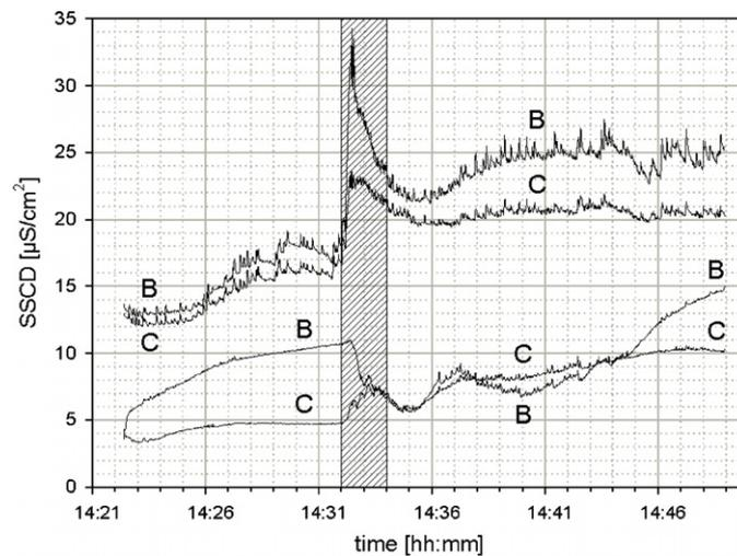
**Figure 8.** Example measurement from one test subject wearing electrode types B and C on the hypothenar (upper plots) and the T9 site. The hatched area indicates the 2 min exercise interval.
