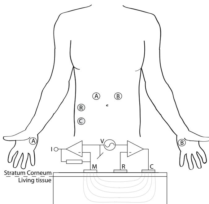
**Figure 1.** Measuring principle, electrode configuration and electrode placement for this study.
