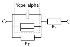
**Figure 2.** The Cole system electrical equivalent model with the components  $R_s$ , a resistor in series with a parallel combination of the resistor  $R_p$  and a constant phase element (CPE). The CPE is characterized by its admittance  $Y_{cpe}$  and its alpha( $\alpha$ ) exponent ( $Y_{cpe} = G_1(\omega\tau)^\alpha$ ).
