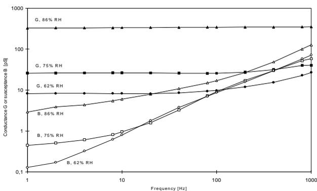
**Fig. 6** Electrical conductance (G) and susceptance (B) of 100 hair fibres in parallel as a function of frequency
