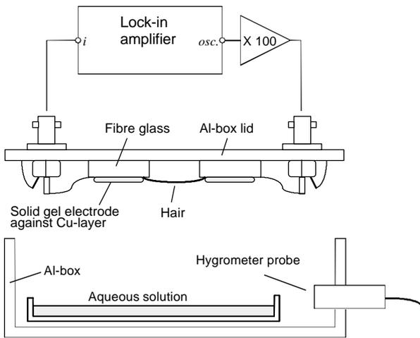
**Fig. 2** Measuring assembly under the lid of an aluminium box
