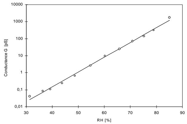
**Fig. 7** Electrical conductance of 50 hair fibres as a function of RH at 1Hz. Circles are measured values and line is logarithmic regression
