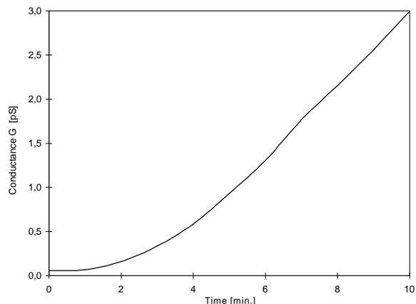
**Fig. 4** Electrical conductance of 100 hair fibres in parallel after a sudden step in RH from 30% to 75% (First 10 min of Fig. 3)
