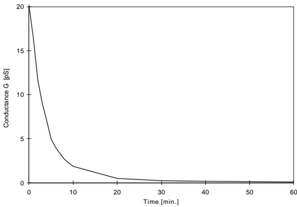
**Fig. 5** Electrical conductance of 100 hair fibres in parallel after a sudden drop in RH from 75% to 30%
