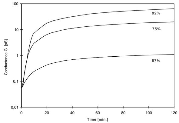
**Fig. 3** Electrical conductance of 100 hair fibres in parallel after a sudden step in RH from 30% to 57%, 75% and 82%
