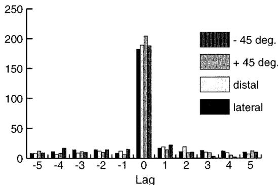
Fig. 7. Number of cross-correlation maxima found in the susceptance measurements at different lags and for different direction of vehicle movement.
