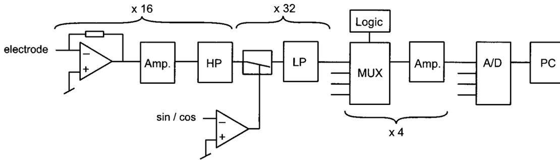
Fig. 3. Block diagram showing the measuring system. Number of parallel elements is indicated.
