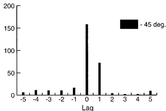
Fig. 8. Number of cross-correlation maxima found in the susceptance measurements at different lags for vehicle movement in  $-45^\circ$  on lateral direction, after introducing an artificial line in the data.
