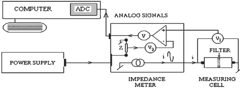
FIG. 1. The Microfiltrimeter block diagram.
