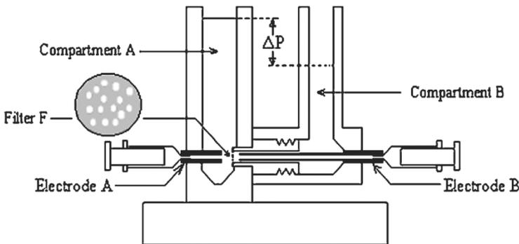
FIG. 2. Schematic diagram of the measuring cell.
