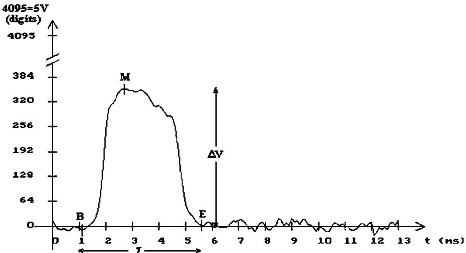
FIG. 3. A typical elementary signal generated by the Microfiltrimeter.
