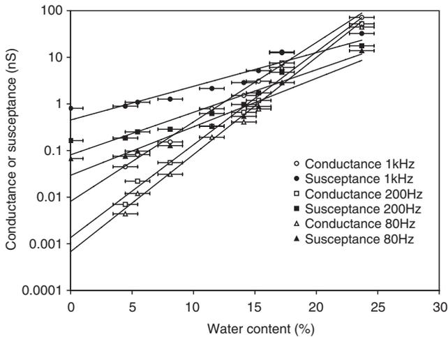
Fig. 5. Conductance and susceptance of nail as a function of frequency and absolute water content. Points represent measured values and lines represent logarithmic regression.
