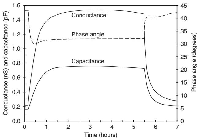
Fig.1. Conductance and capacitance for a piece of toenail after introducing a step in relative humidity from 54% to 68% and back to 54% again. Measured with 100 mV at 200 Hz.
