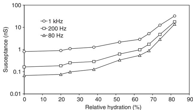
Fig.4. Susceptance of three pieces of nail in series as a function of frequency and relative humidity.
