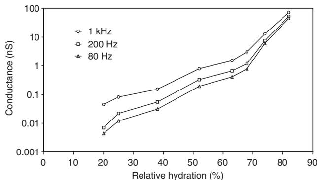
Fig.3. Conductance of three pieces of nail in series as a function of frequency and relative humidity.
