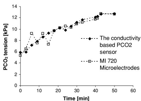
**Figure 10.** Example of an *ex vivo* testing with the conductivity based  $PCO_2$  sensor compared to Stow–Severinghaus sensor.
