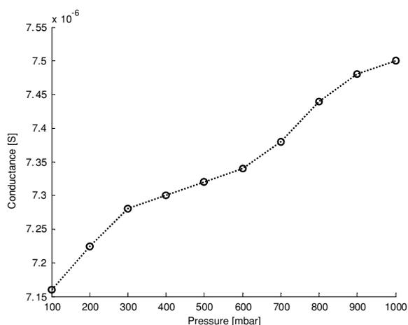
**Figure 9.** Conductance of the sensor as the function of external static pressure.
