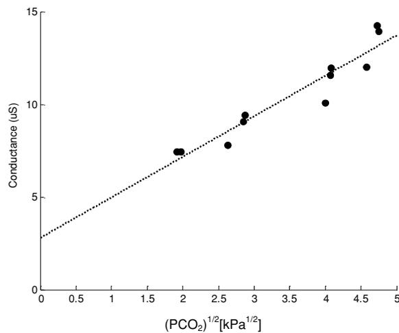
**Figure 6.** Calibration plot of the sensor showing measured conductance versus  $(PCO_2)^{1/2}$ .
