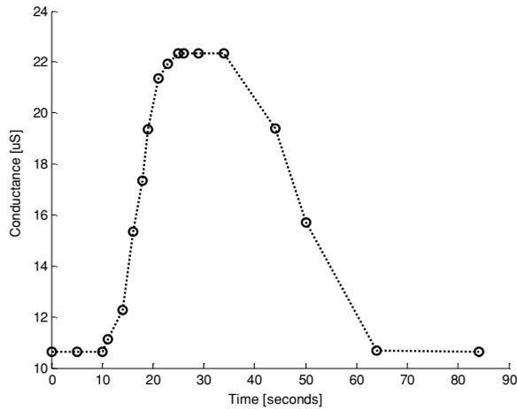
Figure 7. Typical response time with a step from 10 to 20 kPa CO<sub>2</sub> gas tensions.
