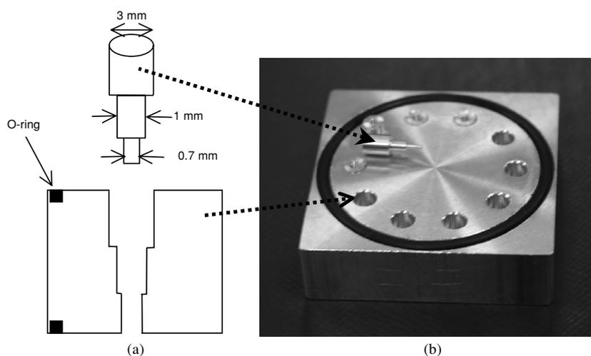
**Figure 4.** (a) The side view drawing of the molding tool and (b) the actual photograph of the molding tool and the pins. The O-ring makes a sealing between the top and bottom plates during the molding.
