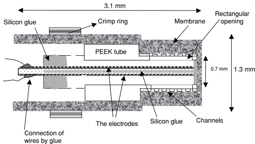
**Figure 1.** Drawing of the  $PCO_2$  sensor assembled with three components, PEEK cylinder, polysiloxane membrane and the electrode assembly with wires glued at the rear end.
