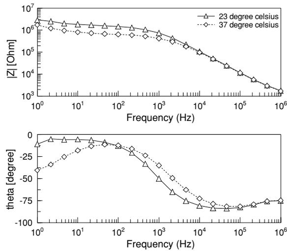
Figure 8. Measured complex impedance as a function of frequency with temperatures at 23 °C and 37 °C.
