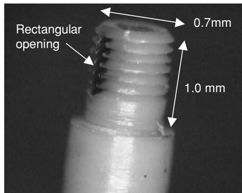
**Figure 3.** Photograph of the sensor inner part before the assembly of the polyimide foil. The inner part is made of a turned PEEK rod with rectangular openings drilled by the excimer laser ablation.
