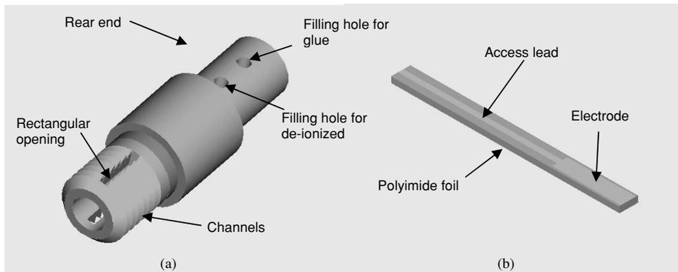
**Figure 2.** The drawings of sensor inner parts without the membrane, (a) PEEK cylinder and the circular ring channels, (b) electrode assembly with polyimide foil covered with gold layer after laser patterning.
