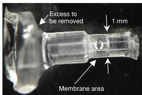
**Figure 5.** Picture of the de-molded membrane before the molding excess was removed.
