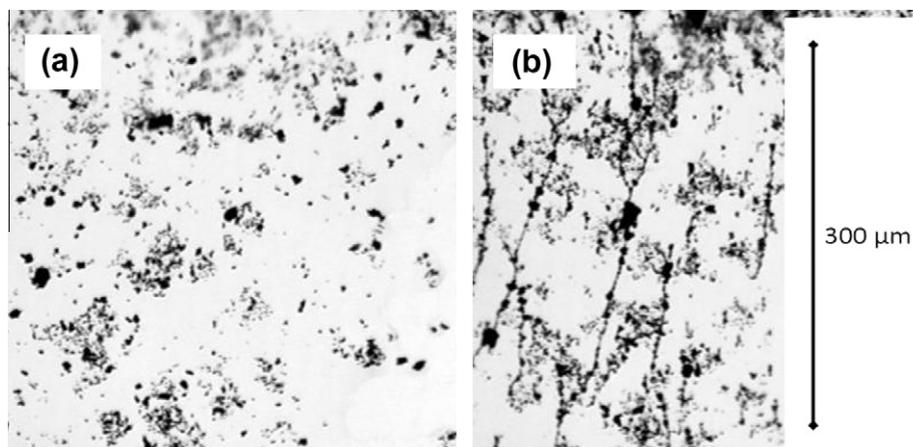
**Fig. 5.** Optical micrographs of aligned silver particles over an electrode distance of 1 mm. 0.25% vol. (a) Isotropic and non-conducting mixture. (b) Mixture after electric field alignment of 1 min, generating conductive wires in-plane. Both images were taken in the transmission geometry.
