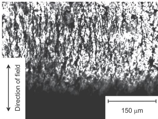
Fig. 6. Side view optical images of aligned silver particles. The particle loading in the polymer was 0.5 vol.%
