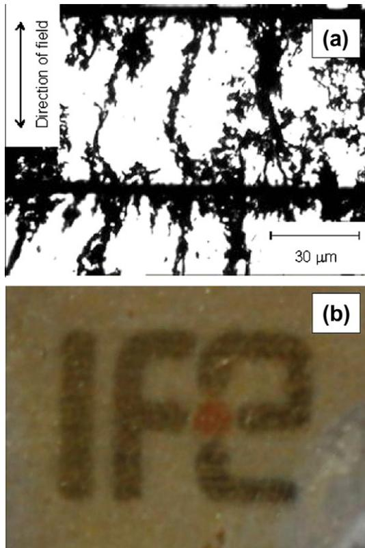
**Fig. 4.** Top view optical images of aligned particles (a). Silver particle loading in the polymer was 0.5 vol.%. The horizontal, black bars are the alignment electrodes. Top view photography (b) of the in-plane aligned sample in (a). The text visible through the sample was about 0.5 cm wide. Both images were taken in the transmission geometry.
