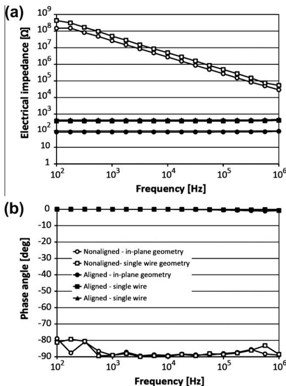
Fig. 7. (a) Absolute value of the electrical impedance,  $Z$ , and (b) phase angle of the studied silver filled adhesives. The open markers correspond to the non-aligned samples, whereas the filled markers correspond to the aligned 0.15 vol.% single wires as well as a 0.4% aligned in-plane, macroscopic sheet (filled circle).
