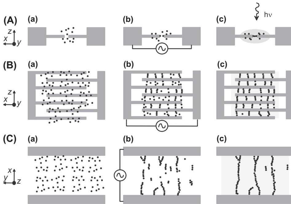
**Fig. 1.** Schematics of the set-ups used for preparations of conductive adhesives with aligned silver wires. (A) Refers to the single wire generation from an isotropic, (a) 0.15 vol.% silver mixture through, (b) electric field alignment and (c) curing of polymer by UV light. (B) Refers to in-plane alignment, creating conductive sheets through the same procedure. (C) Refers to out-of-plane alignment.
