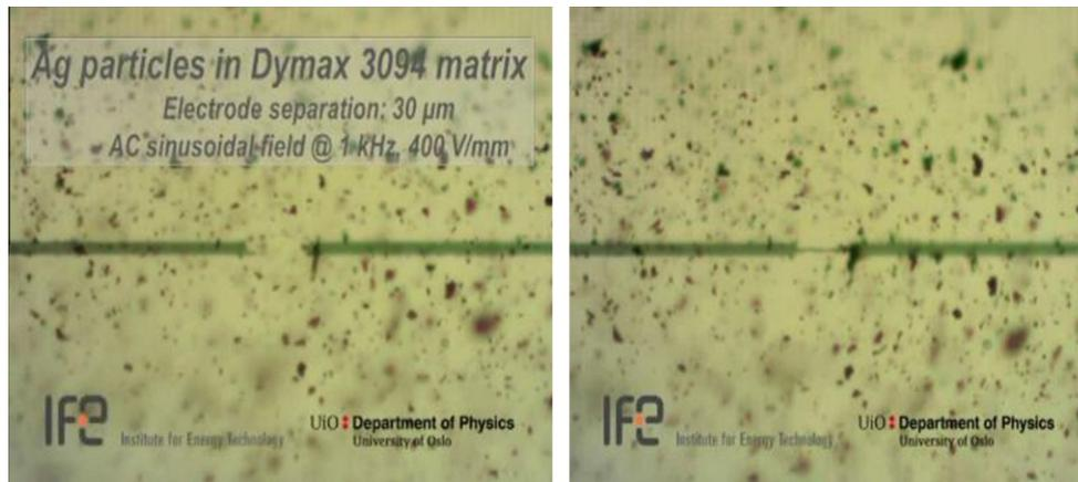
**Fig. 2.** Snapshots of a video clip of silver particles alignment, resulting in a single wire. The left image was taken before, whereas the right after 15 s of alignment. The distance between the electrode tips were 30  $\mu\text{m}$ , the volume filler fraction 0.15%. The electric field strength was 4 kV/cm.
