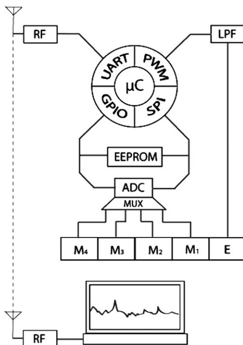
**Figure 1.** Measurement system with four measuring channels, data storage and host communication.
