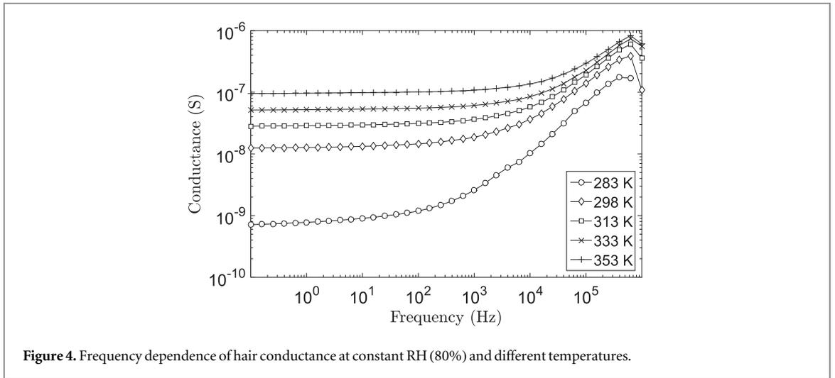
Figure 4. Frequency dependence of hair conductance at constant RH (80%) and different temperatures.
