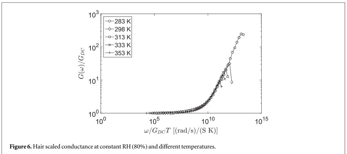
Figure 6. Hair scaled conductance at constant RH (80%) and different temperatures.
