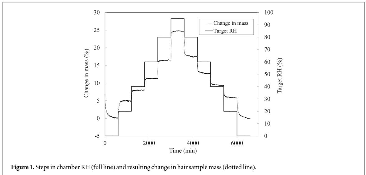
Figure 1. Steps in chamber RH (full line) and resulting change in hair sample mass (dotted line).
