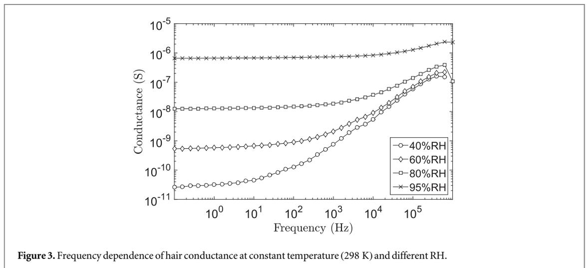
Figure 3. Frequency dependence of hair conductance at constant temperature (298 K) and different RH.
