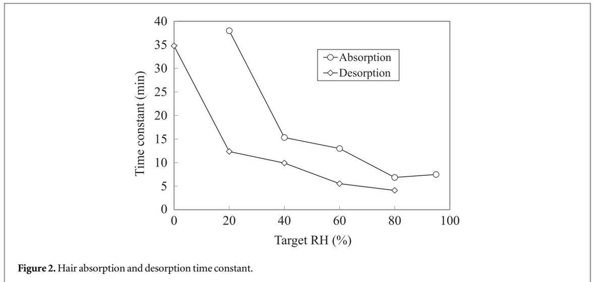
Figure 2. Hair absorption and desorption time constant.
