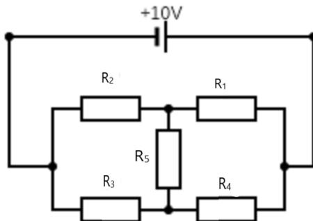
$R_1 = 2 \Omega$ ,  $R_2 = 8 \Omega$ ,  $R_3 = 5 \Omega$ ,  $R_4 = 5 \Omega$ ,  $R_5 = 3000 \Omega$ . The source of voltage is 10 V and it has positive pole to the right in the figure above. Approximately how large is the current through the resistor  $R_5$ ?
