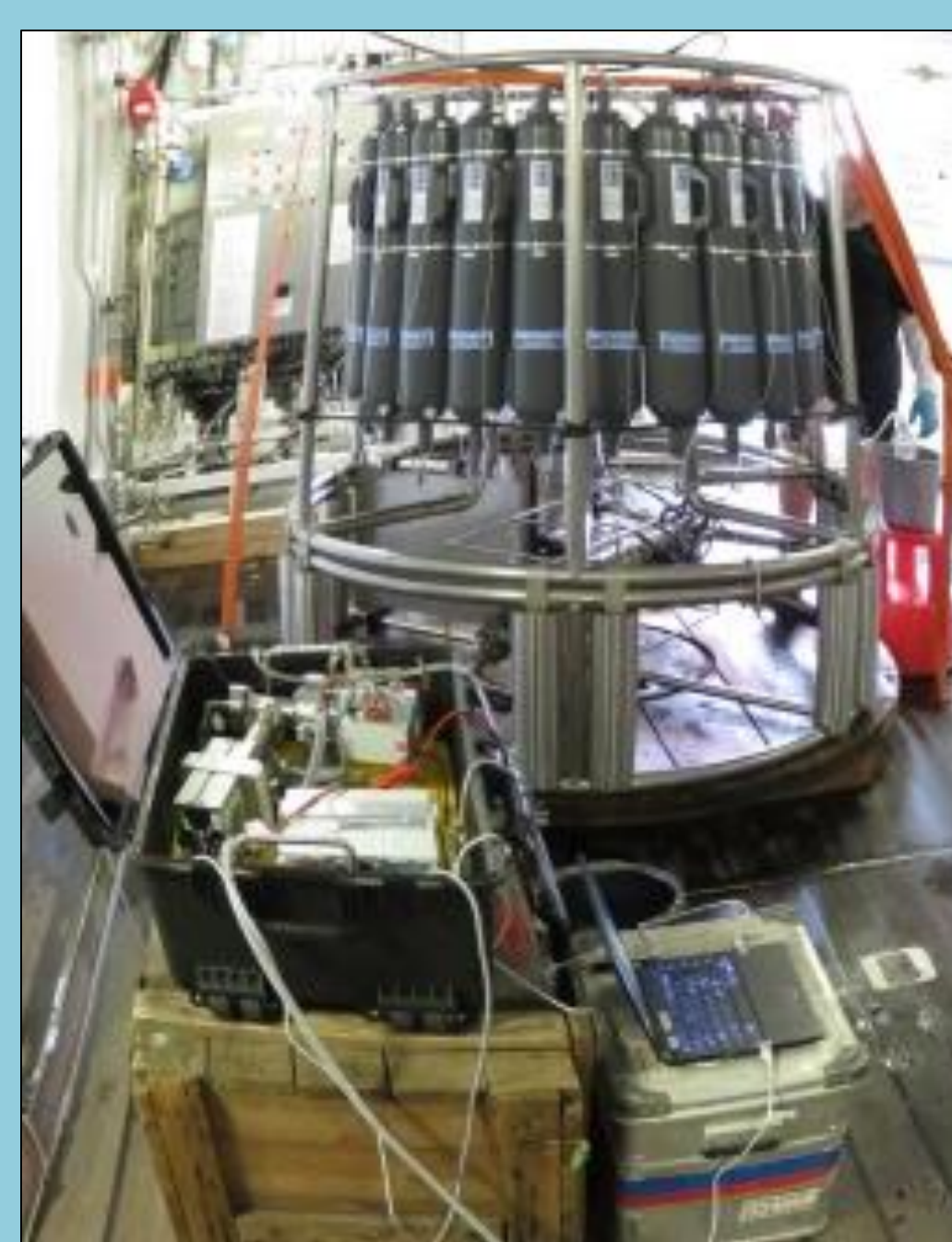
Fig. 2 A: The Mini-Ruedi set-up [1] B: The Mini-Ruedi instrument in operation on oceanic expeditions. The portable GE-MIMS system was installed on RV Sonne during the SO241 expedition in the Guyamas Basin, Gulf of Mexico to analyse gas seeping from the ocean floor [2]. The instrument was connected over small membrane modules with the Niskin bottles of a standard oceanographic rosetta. This set-up allowed to determine the dissolved gas conc.(e.g., He, Ar, Kr, CH 4 , CO 2 ) in sampled ocean water on-line and on-board [1, 2]. C: Fascination of the Mini Ruedi. Photo: M.S. Brennwald. References: [1] Brennwald, M. S., Schmidt, M., Oser J. & Kipfer, R. (2016) A portable and autonomous mass spectrometric system for on-site environmental gas analysis. Environ. Sci. Technol. 50(24), 13455-13463. [2] Berndt, C., Hensen, C., Mortera-Gutierrez, C., Sarkar, S., ... & Muff, S. (2016). Rifting under steam—How rift magmatism triggers methane venting from sedimentary basins. Geology, 44(9), 767-770.
