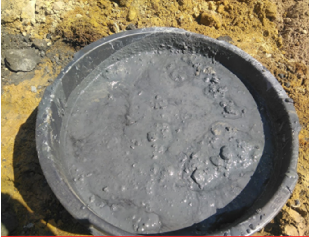
Fluidized till from Gravarhovda, Dagali, with natural water saturation.
