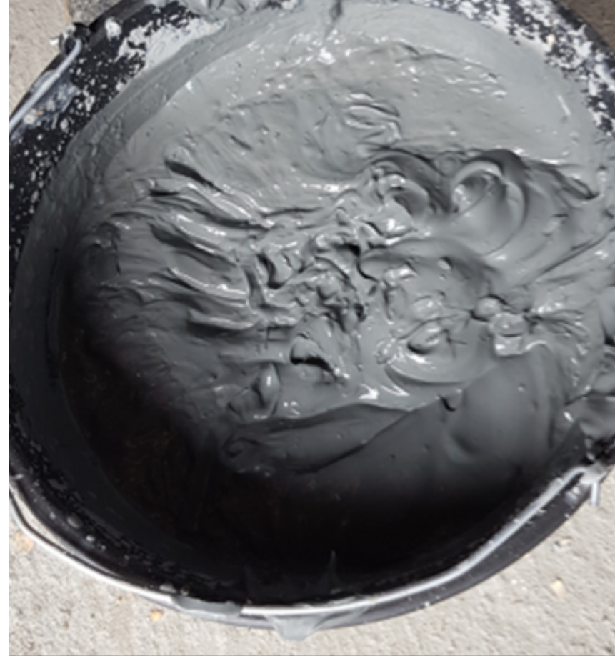
Quick marine clay from Levanger, Mid-Norway.
