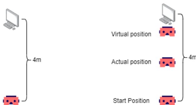
Figure 12: The user wishes to approach the computer 4 meters ahead. The translation scale is 2.0. The user only moves 2 meters in the real world, and has been displaced 4 meters in the virtual world
