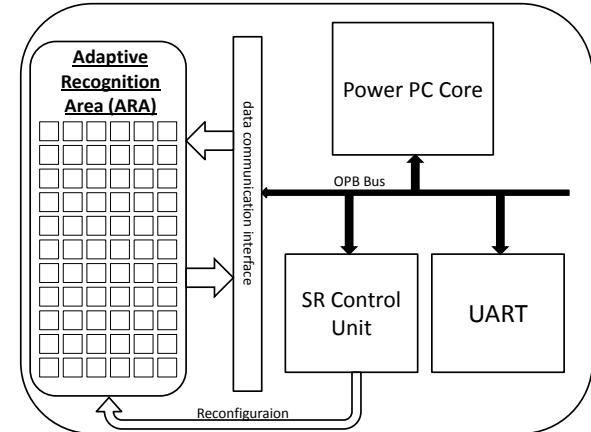
Figure 4: The overall structure of the on-chip system.
