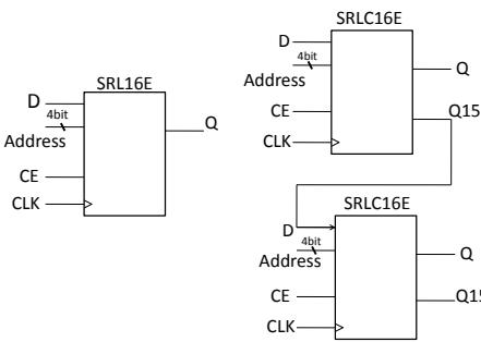
Figure 7: Shift registers used in the system
