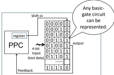
Figure 6: Shift operation in adaptive basic-gate circuit (ABG circuit) with PPC.
