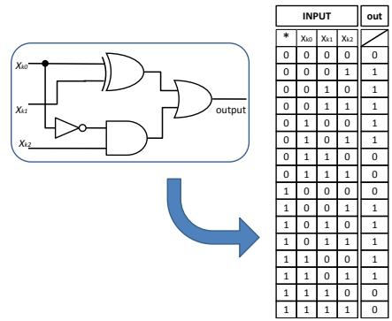
Figure 5: A LUT that represents a basic-gate circuit.
