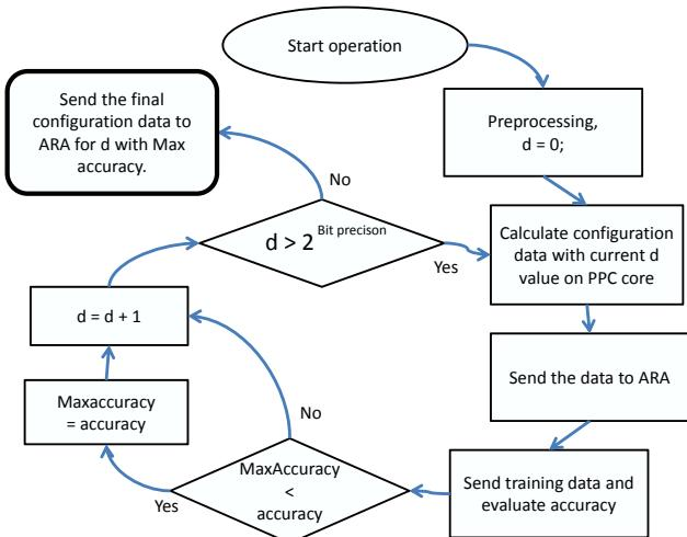
Figure 8: Flowchart of the on-chip adaptive operation.
