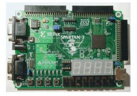
Fig. 2. The Spartan-3 Starter Kit board used in the lab exercises.
