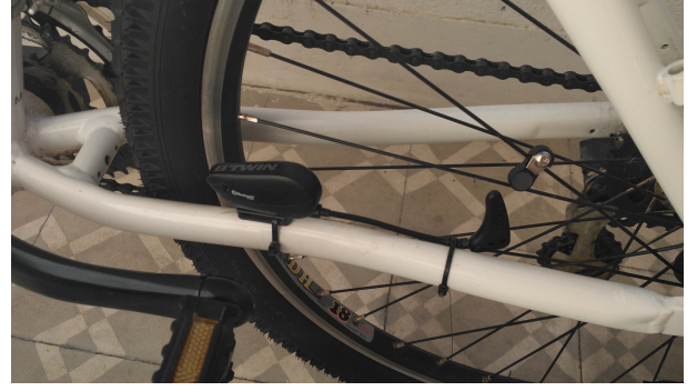
Fig. 2. Biklio bicycle-mounted sensor.
