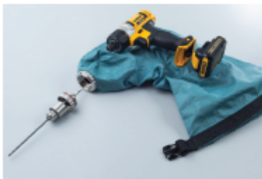
Figure 2 Arbutus Medical Drill Cover System disconnected to show chuck mechanism and liner, with DeWalt drill beside.
