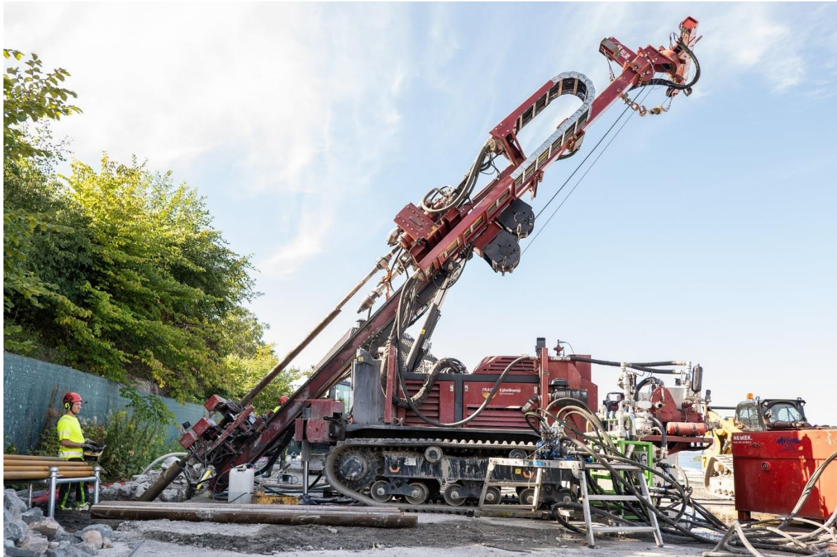
Figure 1. NGI rig for ground investigation
