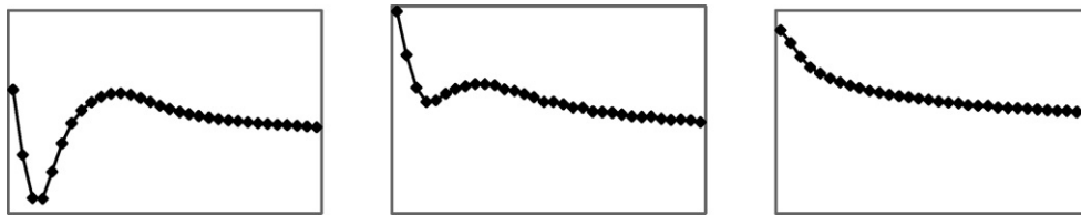
Figure 7 NRT measurement templates. The AutoNRT expert systems correlate a given NRT measurement with these templates to assist classification. Left: Clear ECAP. Middle: ECAP plus stimulus artefact. Right: Stimulus artefact only.
