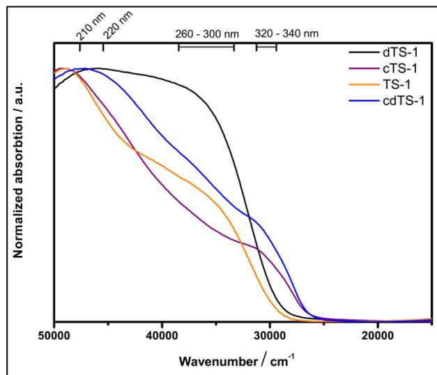
**Figure 1.** UV-Vis spectra of TS-1 and its mesoporous derivatives
