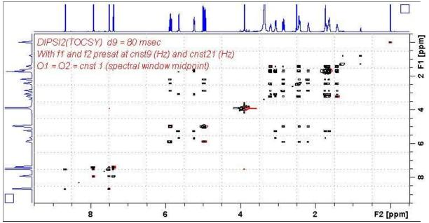
600 MHz **Dipsi2bfprf1bfprf2** spectrum of quinine in D<sub>6</sub>-DMSO with the HOD and DMSO lines at 3.38 ppm and 2.5 ppm suppressed. The spectrum is centered at 4.5 ppm.
