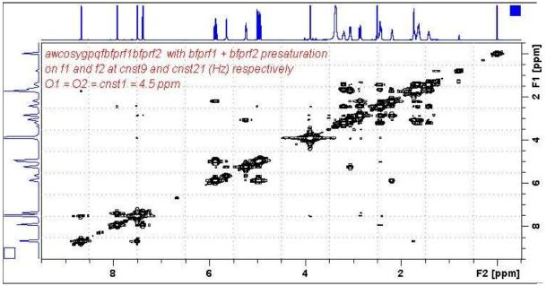
600 MHz Cosybfprf1bfprf2 spectrum of quinine in D<sub>6</sub>-DMSO with the HOD and DMSO lines at 3.38 ppm and 2.5 ppm suppressed. The spectrum is centered at 4.5 ppm.
