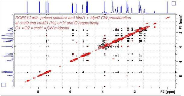
600 MHz Roesy2bfprf1bfprf2 spectrum of quinine in D<sub>6</sub>-DMSO with the HOD and DMSO lines at 3.38 ppm and 2.5 ppm suppressed. The spectrum is centered at 4.5 ppm.
