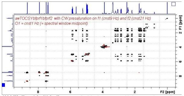
600 MHz **Tocsybfprf1bfprf2** spectrum of quinine in D<sub>6</sub>-DMSO with the HOD and DMSO lines at 3.38 ppm and 2.5 ppm suppressed. The spectrum is centered at 4.5 ppm.
