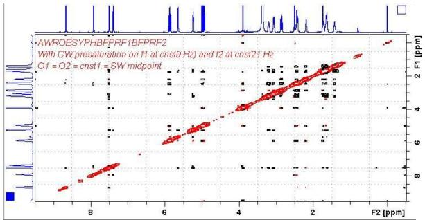
600 MHz **Roesybfprf1bfprf2** spectrum of quinine in D<sub>6</sub>-DMSO with the HOD and DMSO lines at 3.38 ppm and 2.5 ppm suppressed. The spectrum is centered at 4.5 ppm.
