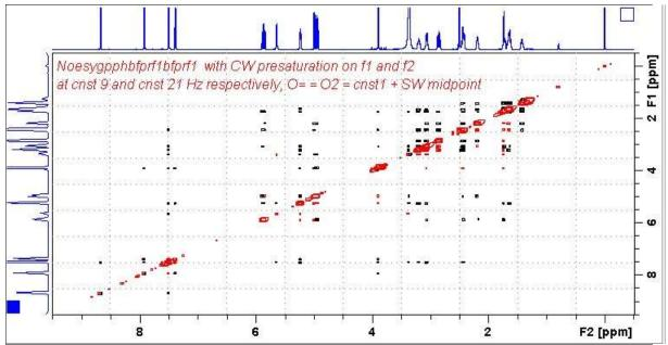
600 MHz **Noesybfprf1bfprf2** spectrum of quinine in D<sub>6</sub>-DMSO with the HOD and DMSO lines at 3.38 ppm and 2.5 ppm suppressed. The spectrum is centered at 4.5 ppm.
