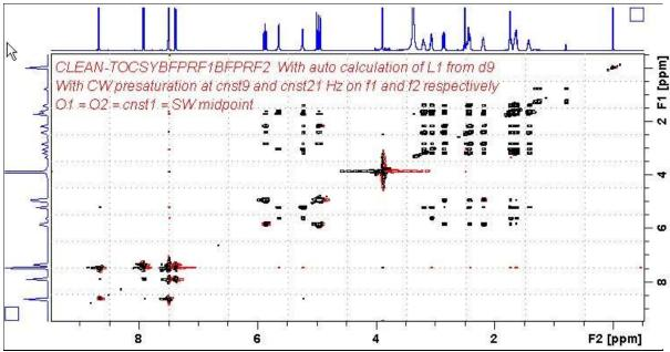
600 MHz Clean-tocsybfprf1bfprf2 spectrum of quinine in D<sub>6</sub>-DMSO with the HOD and DMSO lines at 3.38 ppm and 2.5 ppm suppressed. The spectrum is centered at 4.5 ppm.
