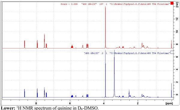
Upper: <sup>1</sup>H NMR spectrum with CW presaturation of the HOD (3.37 ppm) and DMSO (2.5 ppm) lines.
