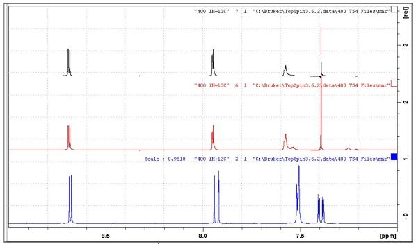
**Lower:** The 7-9 ppm region of the <sup>1</sup>H NMR spectrum of quinine in D<sub>6</sub>-DMSO. **Center:** 7-9 ppm region with homonuclear decoupling at 7.39 ppm during FID acquisition. **Upper:** 7-9 ppm region with homonuclear decoupling at 7.39 ppm during D1 + FID acquisition.
