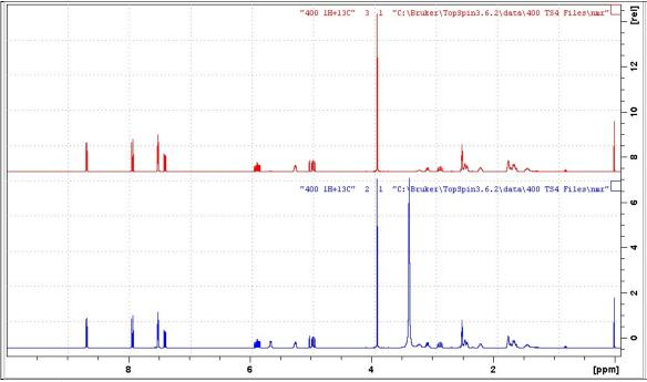
**Lower:** <sup>1</sup>H NMR spectrum of quinine in D<sub>6</sub>-DMSO. **Upper:** <sup>1</sup>H NMR spectrum with CW presaturation of the HOD line at 3.37 ppm.
