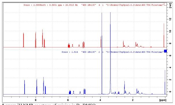
**Lower:** <sup>1</sup>H NMR spectrum of quinine in  $D_6$ -DMSO. **Upper:** <sup>1</sup>H NMR spectrum with ES suppression of the HOD line at 3.37 ppm. The ES spectrum is slightly offset relative to the 1H NMR spectrum.
