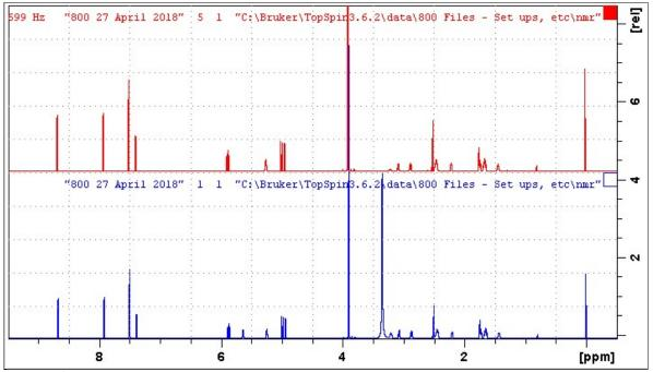
**Lower:** <sup>1</sup>H NMR spectrum of quinine in D<sub>6</sub>-DMSO. **Upper: NOESYPR1D** spectrum with CW presaturation of the HOD line at 3.37 ppm
