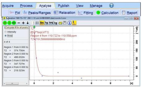
The plot's upper title line correctly has  $T_2$ , but the  $T_1$  equation incorrectly appears below it. This is a long standing Topspin bug.
