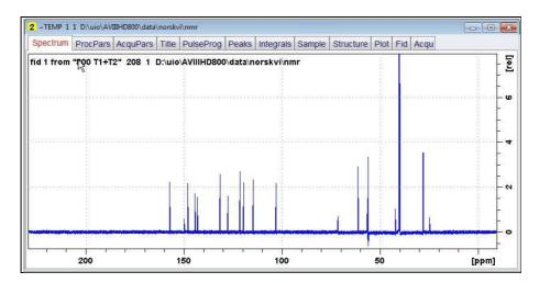
**10)** Type **edp** (enter) and note the phase constants for this spectrum. The **PHC1** angle may be in the range -500 to -700 degrees.
