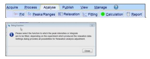
**24**) When the **Fitting** function message screen is closed a panel with **Relaxation parameters** (split into two screen captures below) will appear.
