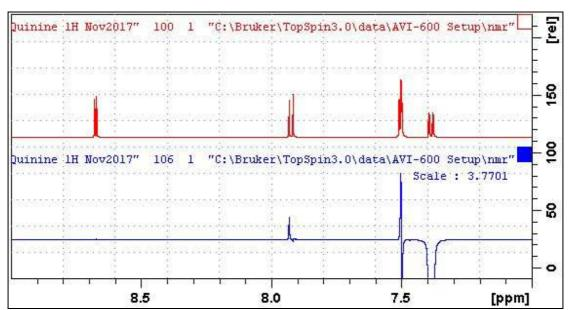
**Upper:** 7-9 ppm region of the 600 MHz <sup>1</sup>H NMR spectra of quinine in D<sub>6</sub>-DMSO. **Lower:** SELROESY2 spectrum ex the signal at 7.39 ppm. An antiphsase TOCSYartifact peak appears at 7.52 ppm. A weak ROESY correlation, attenuated by a significant antiphaseTOCSY artifact contribution is observed at 7.93 ppm.
