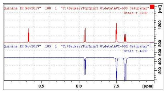
**Upper:** 7-9 ppm region of the 600 MHz <sup>1</sup>H NMR spectra of quinine in D<sub>6</sub>-DMSO. **Lower:** SELROESY spectrum ex the signal at 7.39 ppm. Only negative TOCSY artifact peaks were observed when the SELROESY spectrum was determined d with the **prosol** Table linked PL11 CW spin lock power level.
