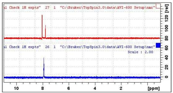
600 MHz **SELHSQC** (*lower*) and **SELHSQCND** (*upper*) spectra determined for quinine in  $D_6$ -DMSO with selective excitation of the  $^{13}$ C signal at 131.6 ppm (O2 = 19857 Hz).
