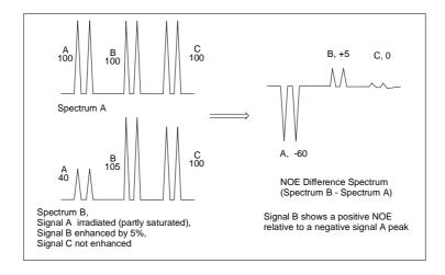
A positive NOE is one in which a positive enhanced peak is observed relative to a **negative irradiated peak** in a 1D-SELNOESY experiment, or a **negative diagonal peak** in a 2D-NOESY experiment.
