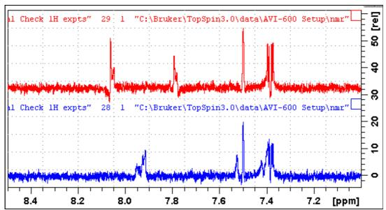
Expansions of the 7-8.5 ppm regions of the 600 MHz **SELHSQC-DIPSI2** (*lower*) and **SELHSQCND-DIPSI2** (*upper*) spectra determined for quinine in D<sub>6</sub>-DMSO with selective excitation of the  $^{13}$ C signal at 131.6 ppm (O2 = 19857 Hz). The  $^{1}J$  correlated proton signal occurs at 7.95 ppm.
