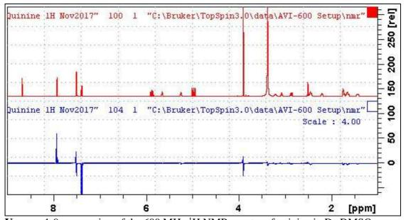
**Upper:** 1-9 ppm region of the 600 MHz <sup>1</sup>H NMR spectra of quinine in D<sub>6</sub>-DMSO. **Lower:** SELNOSY spectrum ex the signal at 7.39 ppm. The signal at 7.51 ppm is an antiphase COSY artifact peak.
