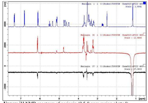
**Upper:** <sup>1</sup>H NMR spectrum of naringin (0.5-8 ppm region plotted). **Center:** SELROESY spectrum ex the methyl signal at 1.2 ppm. **Lower:** SELNOESY spectrum ex the methyl signal at 1.2 ppm.
