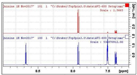
**Lower:** 7-9 ppm region of the 600 MHz <sup>1</sup>H NMR spectra of quinine in D<sub>6</sub>-DMSO. **Upper:** Power mode processed SELCOSY spectrum ex the signal at 7.39 ppm.
