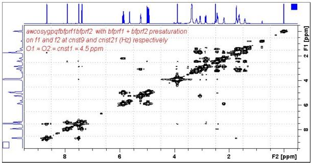
AVI-600 **Cosybfprf1bfprf2** spectrum of quinine in  $D_6$ -DMSO with the HOD and DMSO lines at 3.38 ppm and 2.5 ppm suppressed. The spectrum is centered at 4.5 ppm (O1 = O2 = CNST 1 = 2700.59 Hz).
