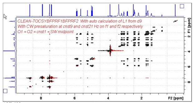
AVI-600 Clean-tocsybfprf1bfprf2 spectrum of quinine in  $D_6$ -DMSO with the HOD and DMSO lines at 3.38 ppm and 2.5 ppm suppressed. The spectrum is centered at 4.5 ppm (O1 = O2 = CNST 1 = 2700.59 Hz).
