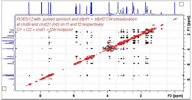
AVI-600 **Roesy2bfprf1bfprf2** spectrum of quinine in  $D_6$ -DMSO with the HOD and DMSO lines at 3.38 ppm and 2.5 ppm suppressed. The spectrum is centered at 4.5 ppm (O1 = O2 = CNST 1 = 2700.59 Hz).
