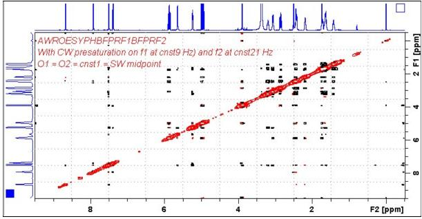
AVI-600 **Roesybfprf1bfprf2** spectrum of quinine in  $D_6$ -DMSO with the HOD and DMSO lines at 3.38 ppm and 2.5 ppm suppressed. The spectrum is centered at 4.5 ppm (O1 = O2 = CNST1 = 2700.59 Hz).
