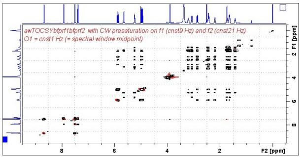
AVI-600 **Tocsybfprf1bfprf2** spectrum of quinine in  $D_6$ -DMSO with the HOD and DMSO lines at 3.38 ppm and 2.5 ppm suppressed. The spectrum is centered at 4.5 ppm (O1 = O2 = CNST1 = 2700.59 Hz).
