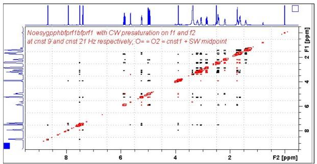
AVI-600 **Noesybfprf1bfprf2** spectrum of quinine in  $D_6$ -DMSO with the HOD and DMSO lines at 3.38 ppm and 2.5 ppm suppressed. The spectrum is centered at 4.5 ppm (O1 = O2 = CNST 1 = 2700.59 Hz).
