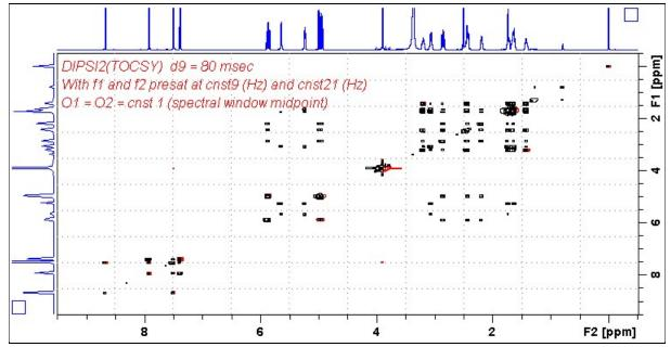
AVI-600 **Dipsi2bfprf1bfprf2** spectrum of quinine in  $D_6$ -DMSO with the HOD and DMSO lines at 3.38 ppm and 2.5 ppm suppressed. The spectrum is centered at 4.5 ppm (O1 = O2 = CNST 1 = 2700.59 Hz).
