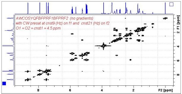
AVI-600 **Cosyqfbfprf1bfprf2** spectrum of quinine in  $D_6$ -DMSO with the HOD and DMSO lines at 3.38 ppm and 2.5 ppm suppressed. The spectrum is centered at 4.5 ppm (O1 = O2 = CNST1 = 2700.59 Hz).
