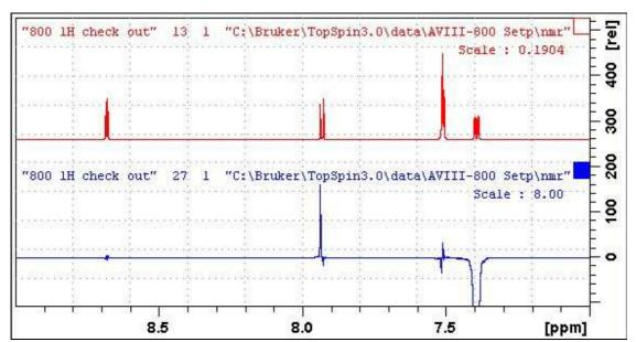
**Upper:** 7-9 ppm region of the 800 MHz  $^{1}$ H NMR spectra of quinine in D<sub>6</sub>-DMSO. **Lower:** SELROESY2 spectrum ex the signal at 7.39 ppm with PLW11 = 8.48 db
