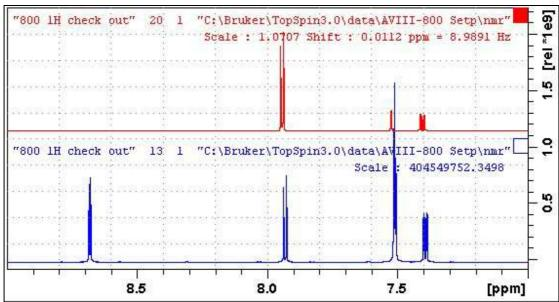
**Lower:** 7-9 ppm region of the 800 MHz <sup>1</sup>H NMR spectra of quinine in D<sub>6</sub>-DMSO. **Upper:** Power mode processed SELCOSY spectrum ex the signal at 7.39 ppm.
