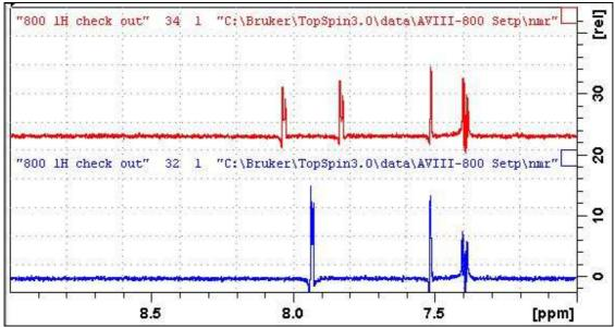
7-9 ppm regions of the **SELHSQC-DIPSI2** (*lower*) and **SELHSQCND-DIPSI2** (*upper*) spectra determined for quinine in D<sub>6</sub>-DMSO with selective excitation of the  $^{13}$ C signal at 131.6 ppm (O2 = 26475 Hz). The  $^{1}J$  correlated proton signal occurs at 7.95 ppm.
