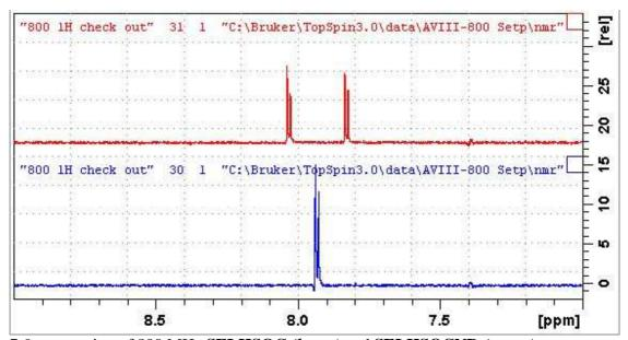
7-9 ppm region of 800 MHz **SELHSQC** (*lower*) and **SELHSQCND** (*upper*) spectra determined for quinine in D<sub>6</sub>-DMSO with selective excitation of the  $^{13}$ C signal at 131.6 ppm (O2 = 26475 Hz). The  $^{1}J$  correlated proton signal occurs at 7.95 ppm.
