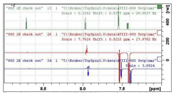
**Upper:** 7-9 ppm region of the 800 MHz  $^{1}$ H NMR spectra of quinine in D<sub>6</sub>-DMSO. **Center:** SELROESY spectrum ex the signal at 7.39 ppm with PLW11 = 20.48 db **Lower:** SELROESY spectrum ex the signal at 7.39 ppm with PLW11 = 8.48 db
