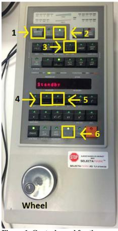
Figure 1. Control panel for the DPX200 instrument (the DPX300 instrument does not have a  $\mathbf{Z}^0$ ).
