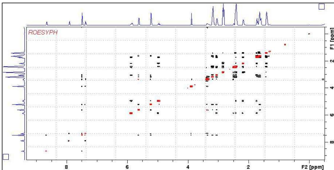
ROESY spectrum of quinine in D<sub>6</sub>-DMSO. The spectrum is centered at 4.5 ppm.
