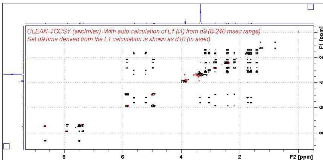
CLEAN-TOCSY spectrum of quinine in D<sub>6</sub>-DMSO. The spectrum is centered at 4.5 ppm.
