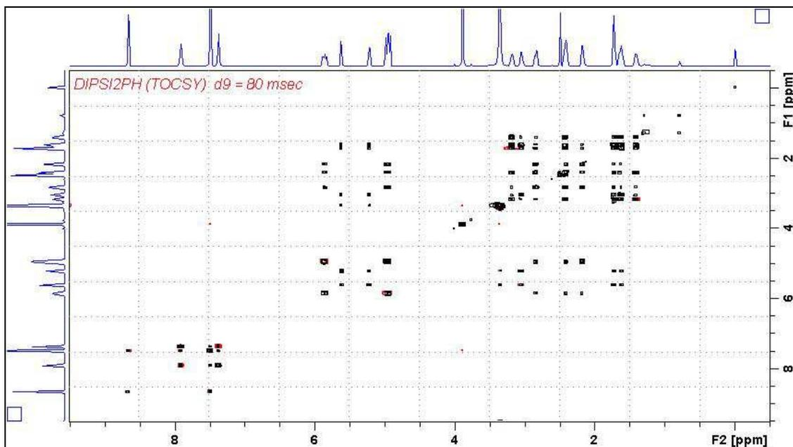
**DIPSI2** spectrum of quinine in D<sub>6</sub>-DMSO. The spectrum is centered at 4.5 ppm.
