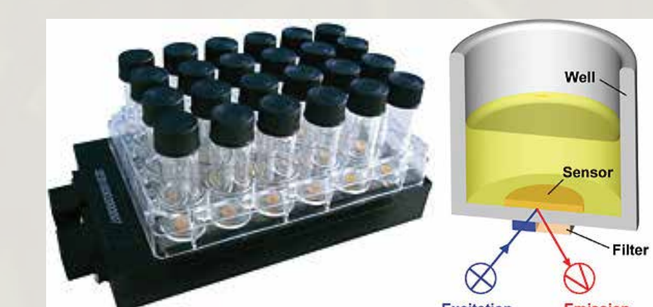
Figure 3: PreSens Sensor®Dish reader system with multiple 5 mL sample vials. Outline of the sensor spot present in each vial. (www.presens.de)
