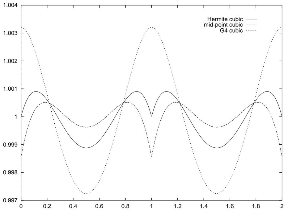
Figure 8. The curvature of the three sixth order approximations of two adjacent 45 degree circular arcs.
