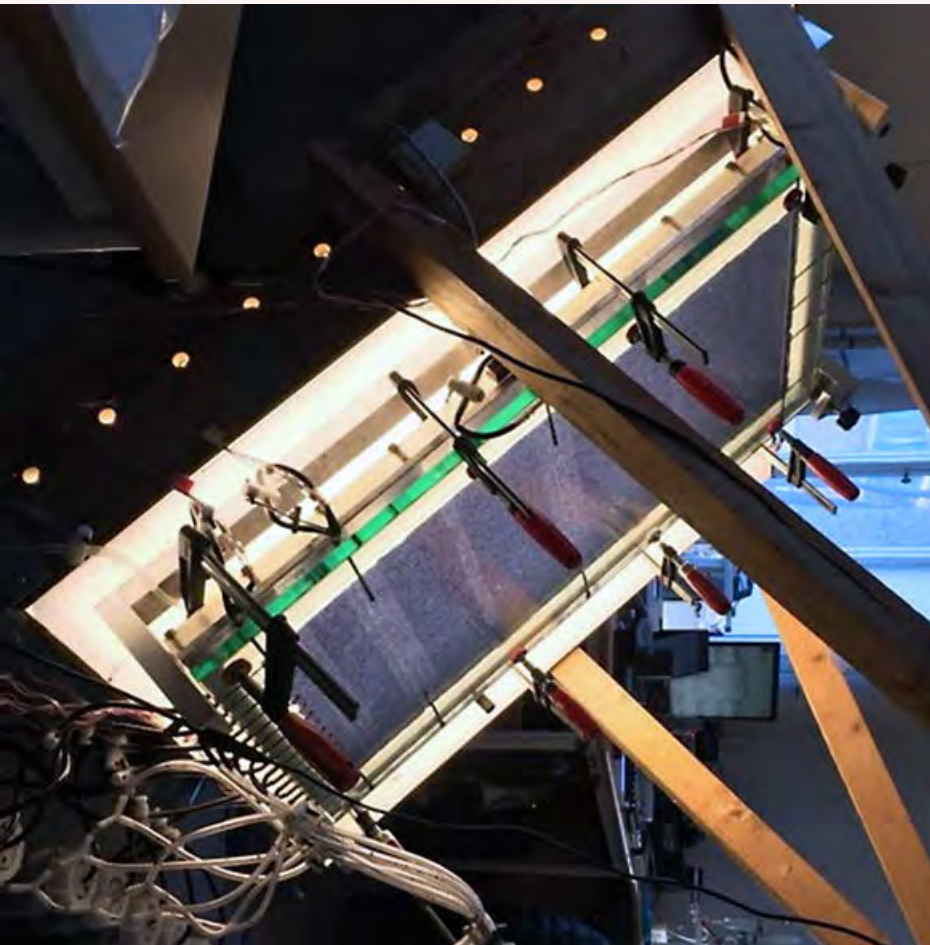
Figure 1: Photograph of the experimental setup, showing the liquid saturated porous Hele-Shaw cell at a 45 degrees tilting angle. The fluids are injected simultaneously into the cell inlet (bottom right) at a constant flow rate, while the outlet (top left) is open to the atmosphere. This tilting angle introduces an approx. 0.7 G gravitational component against the flow direction.
