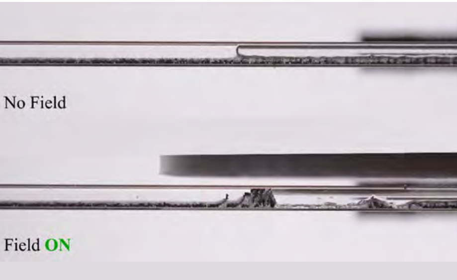
Figure 3: Trigger of the bulldozing instability using ferromagnetic interactions.
