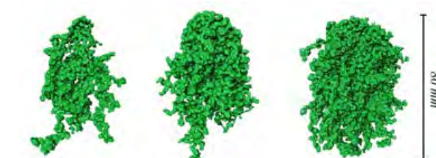
Figure 2: Images of the 3D configuration of a green liquid invading a less dense and less viscous liquid in a porous medium, from the top, captured at percolation. Flow rates increase from left to right. The structures consist of a compact region, surrounded by thin fingers. The compact centers grow with increasing flow rates, and with time.
