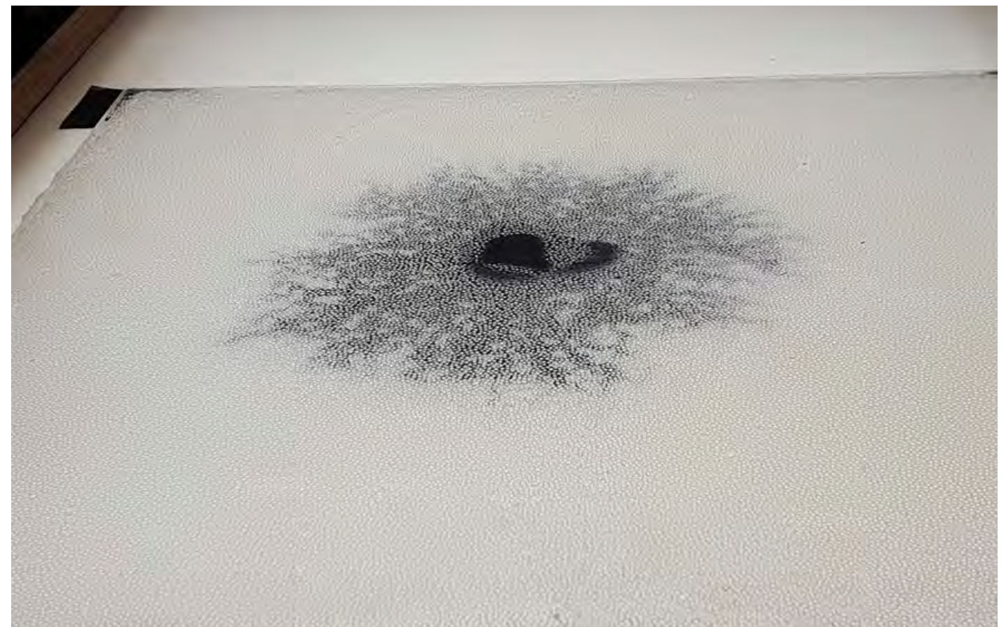
An experiment demonstrating how a source of pollution can permeate through a porous medium. This model gives a direct visualization of what happens for example when polluted water is spilled on the soil.
