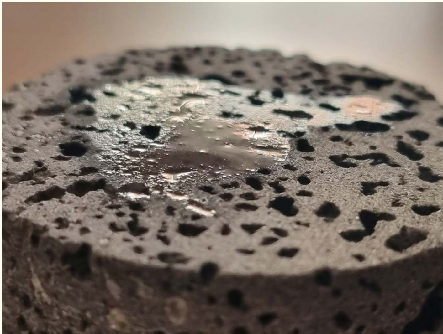
↑ Percolation of reactive fluids within Faroe Island basalt rock can induce carbonate precipitation and alter porosity characteristics.
