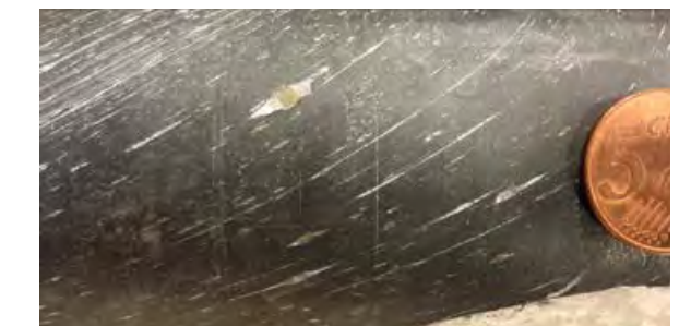
Core sample of highly deformed Alum Shale from the basal décollement of the Caledonian mountain belt
