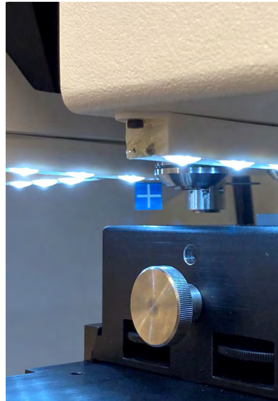
The new nano-indenter at Njord ready to perform mechanical tests on minerals.
