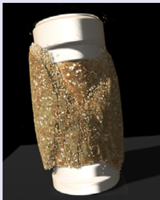
Synchrotron X-ray microtomography scan of a granite core sample deformed until system-size failure performed on beamline BM18 at the European Synchrotron Radiation Facility - Sample dimensions: 10x20 mm. © Benoît Cordonnier.
