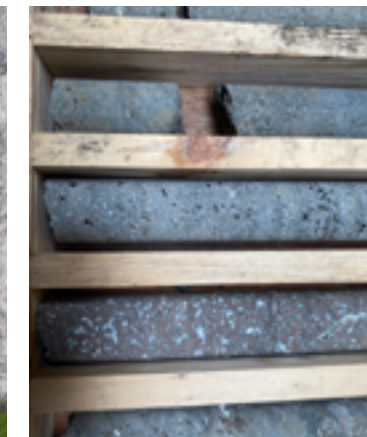
Drill core from the Faroe Islands with basalt flows, some with open pores and some filled with secondary minerals
